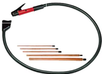
The air carbon-arc process physically removes metal, not chemically as in oxy-fuel cutting. Gouging or cutting occurs when the intense heat of the arc between the carbon electrode and the workpiece melts part of the workpiece. Simultaneously, air passes through the arc quickly enough to blow the molten material away.
