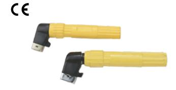
TWIST is an electrode holder completely shielded in the front part. The electrode is positioned at 90 degrees and blocked by rotating the shank. In operation the electrode is completely hidden from the outside reducing the risk of short circuit. Suitable particularly for welding in plain or vertical.
