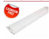
Alloy with high silver content (30%) for assembly of steel/brass/copper. Wide joints in piping, plumbing, climate control and exchangers. Brazing generally at low temperatures.
