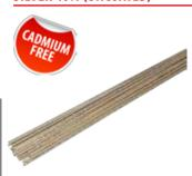
UNCOATED ALLOY WITH 40% SILVER. Alloy for universal use. Brazing, generally at low temperatures, of copper, copper alloys and all kinds of steel, including stainless. Water/gas pipes. Climate control systems.
