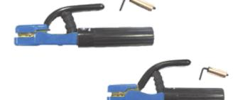
Crocodile electrode holders have a ribbed handle providing a firm grip and good balance. The spring is shielded to prevent damage from spatter and cable fixing is by means of a bolt and copper ferrule (supplied). One of the most popular electrode holders on the market, these are heavy duty.
