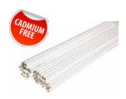
COATED ALLOY WITH 55% SILVER. Alloy with very high silver content for assembly of stainless steel/brass/copper. Especially suitable for medical gases, purified gases and in the food industry. Alloy for universal use. Brazing, generally at low temperatures, of copper, copper alloys and all kinds of steel, including stainless. Narrow joints on stainless steel. Pipes for water/gas and for purified gases or gases destined for food production. Climate control, sanitary fittings.
