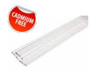
COATED ALLOY WITH 40% SILVER. Alloy for universal use. Brazing, generally at low temperatures, of copper, copper alloys and all kinds of steel, including stainless. Water/gas pipes. Climate control systems.
