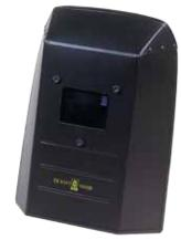
ELETTRA is a hand shield made from cellulose fiber. It is one of the most popular masks for the use with small-medium machines (up to 250A). The new and exclusive "quick glass" fixing system allows a very speedy change of the  $75\times98$  mm lenses without the need of any tool. No metallic rivets are used in the production process!
